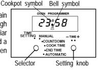
If the oven is switched off on the wall, or there is a loss of power, the clock will stop and you will not be able to use the main oven. When you first switch the electricity supply on, the timer display will flash.
